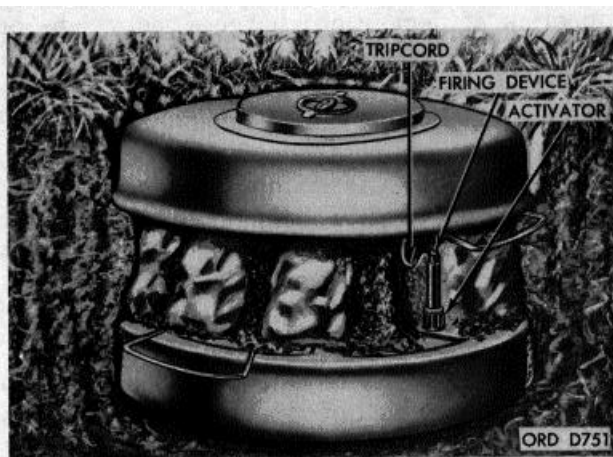
Figure 7-13. Installation of a boobytrapped AT mine.
